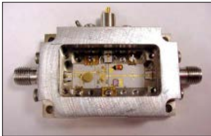
Fig. 1 A 12.5 GHz GaAs FET dielectric resonator oscillator (1.6" × 1" × 0.6"). ▼
