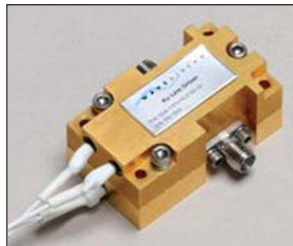
▲ Fig. 5 Compact line driver module used in the DPA.
